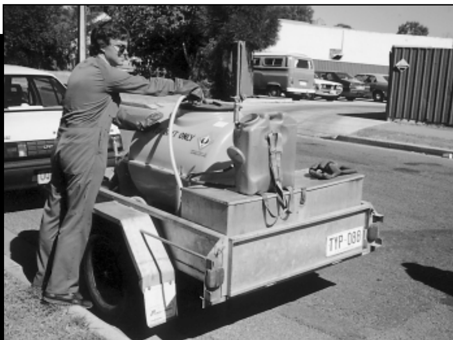
Knapsack sprayer filled from a 400 L bulk tank services a spraying team for one day.
